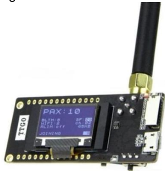
Figura 2. Radio LYLIGO LoRa
