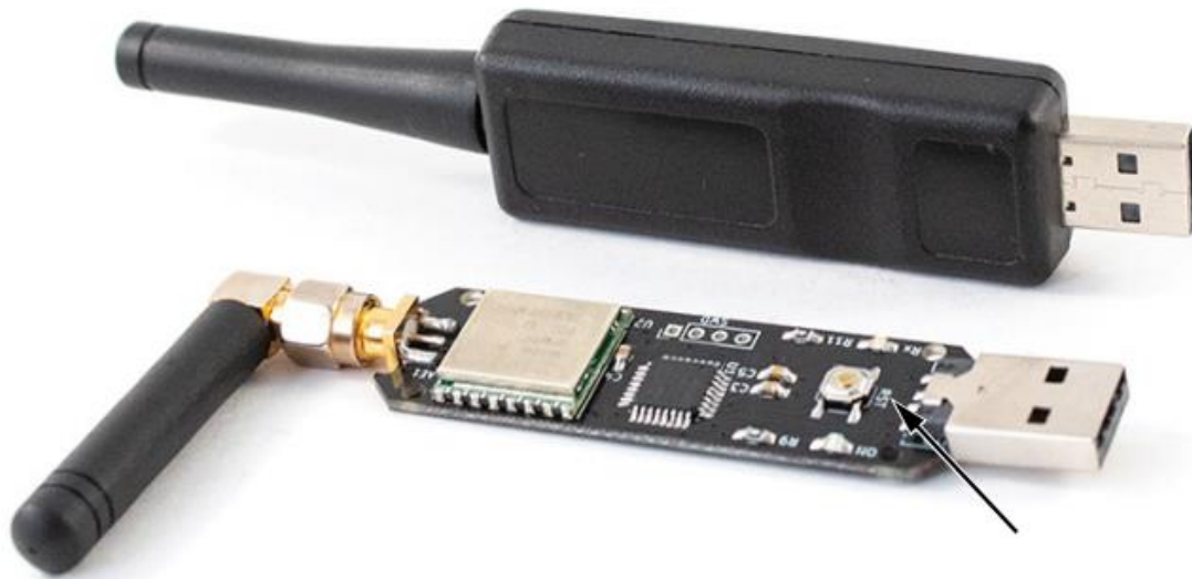
Figure 7-8: CatWAN USB stick, compatible with LoRa and LoRaWAN, es basado en el RFM95 transceiver.
