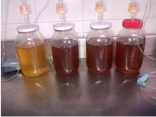
Four glass fermenters (bioreactors) arranged in a row on a laboratory bench. Each fermenter is equipped with a stirrer and aeration system. The liquid inside the fermenters is a dark brown color, indicating the presence of yeast and fermentation products. | Fermentadores a escala de 700 ml con un caudal a 1 vvm a temperatura ambiente a diferentes concentraciones de glicerina |
